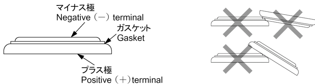
【Battery shape of Coin Manganese Dioxide Lithium Battery】
