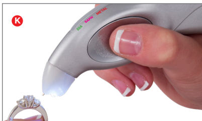
TESTING A MOUNTED STONE
