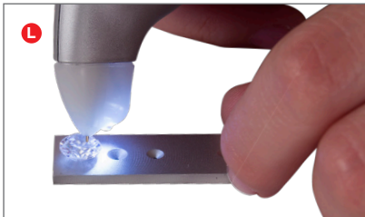
TESTING LOOSE STONES WITH TESTING PLATE
